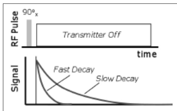
*Excitation and response of the magnetization after a single RF pulse. The 90° pulse rotates the magnetization to the plane perpendicular to  $B_0$ . The signal decays with a relaxation time  $T_2^*$ , the life-time of the FID.*
