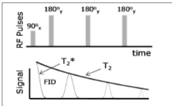
The Carr-Purcell echo pulse sequence for  $T_2$  measurements. The initial  $90^\circ$  pulse rotates the magnetization onto the plane perpendicular to  $B_0$ , and the following sequence of  $180^\circ$  pulses refocuses the static field inhomogeneities while the signal is acquired.
