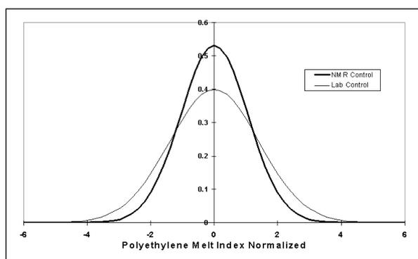
Figure 8: MI consistency improvement with NMR control
