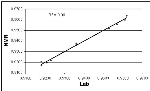
Figure 3: Density calibration using advanced data analysis
