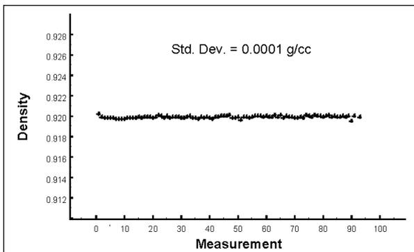
Figure 4: Standard deviation of repeat NMR density analysis
