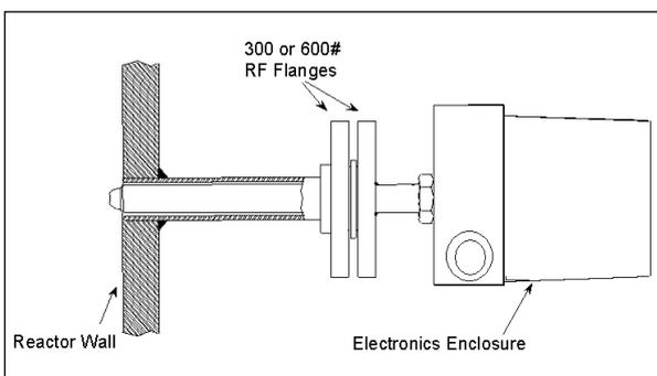
Figure 4: ESM reactor probe and reactor nozzle
