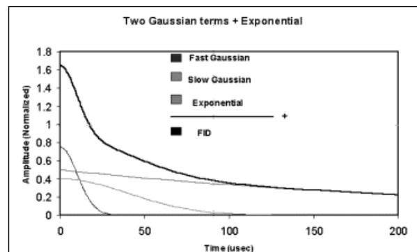
Figure 14: Typical polyethylene FID
