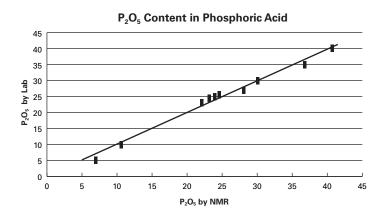
This graph demonstrates a typical performance for the Magneflow NMR technology compared with lab reference data for the analysis of  $P_2O_5$ . In most cases, better quality reference data will result in better calibration results. The Magneflow NMR calibration stability is excellent in the short term, as well as long-term repeatability. A typical performance of <0.05% is expected.
