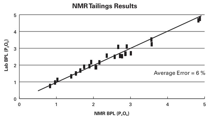
This graph demonstrates a typical performance for the Magneflow NMR technology compared with lab reference data for the  $P_2O_5$  content in tails. In most cases, better quality reference data will result in better calibration results. The Magneflow NMR calibration performance for stability is excellent in both the short term as well as long-term repeatability. A typical long-term repeatability of <0.05% is expected.
