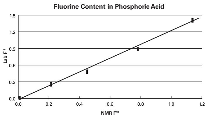
This graph demonstrates a typical performance for the Magneflow NMR technology compared with lab reference data for the analysis fluorine content in phosphoric acid. In most cases, better quality reference data will result in better calibration results. The Magneflow NMR calibration performance is excellent in the short term, as well as long-term repeatability. A typical performance of 0.05% is expected.
